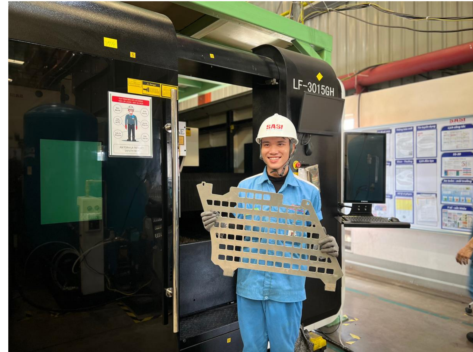
Sheet metal laser cutting Power: 6KW, 12KW Length: 3m
