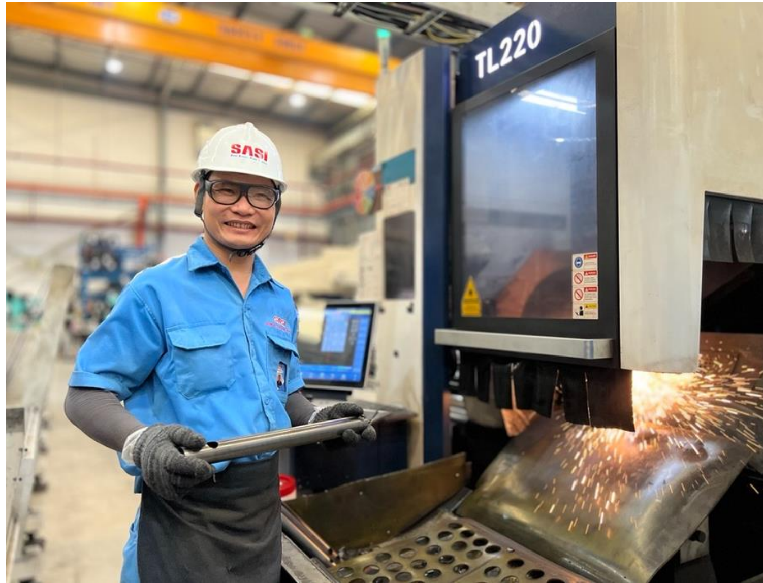
Tube laser cutting Power: 12KW Length: 6m
